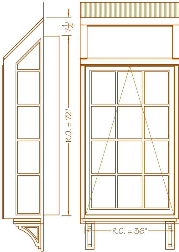
3060A SLEEVE MOUNT WITH 16" PROJECTION (SHOWN WITH SUGGESTED SIMULATED COLONIAL DIVIDED LITES)
