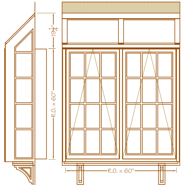
5060A SLEEVE MOUNT 16" PROJECTION WITH 12" SHORTER R.O. (SHOWN WITH SUGGESTED SIMULATED COLONIAL DIVIDED LITES)
